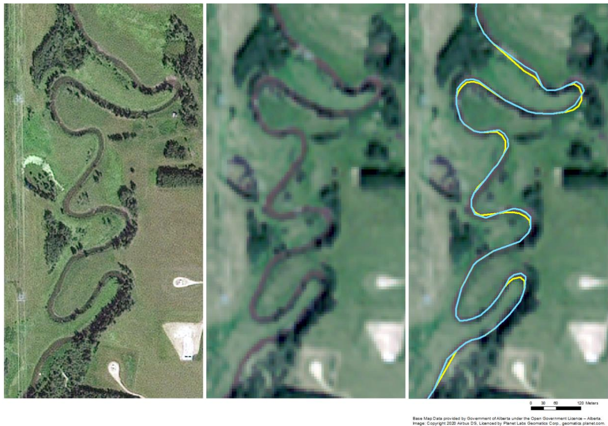
Figure 3. Example of the spatial inaccuracies associated with stream boundaries, where the location of the stream center line does not match the actual location of the stream and exceeds the 5 m accuracy tolerance in the SPOT imagery. In this example, the yellow lines represent the location of the streamline from the provincial data and the blue line represents the manually edited location of the new stream center line.
